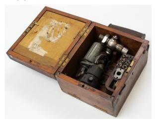
**1299** Valve testing machine for steam engines
